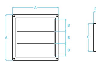
**Please Note:** Being constructed from Polypropylene, our vents do not comply to a BAL Rating and should not be used in Bushfire Zone. It is recommended that a qualified Tradesperson is used to install the Plastic Gravity Louvre Vent and any through the wall ventilation.
